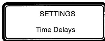
④ You can press the right arrow key to see the other time delay menus (as shown below). An overview explanation of each setting is listed below.
